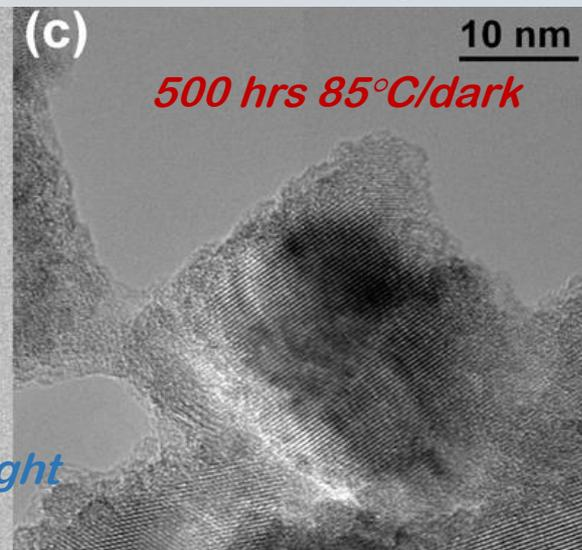
**Formation and growth of an insoluble degradation layer on  $TiO_2$  favored by temperature and ageing time  $\rightarrow$  SEI layer using Pelled nomenclature (Solid Electrolyte Interphase)**
