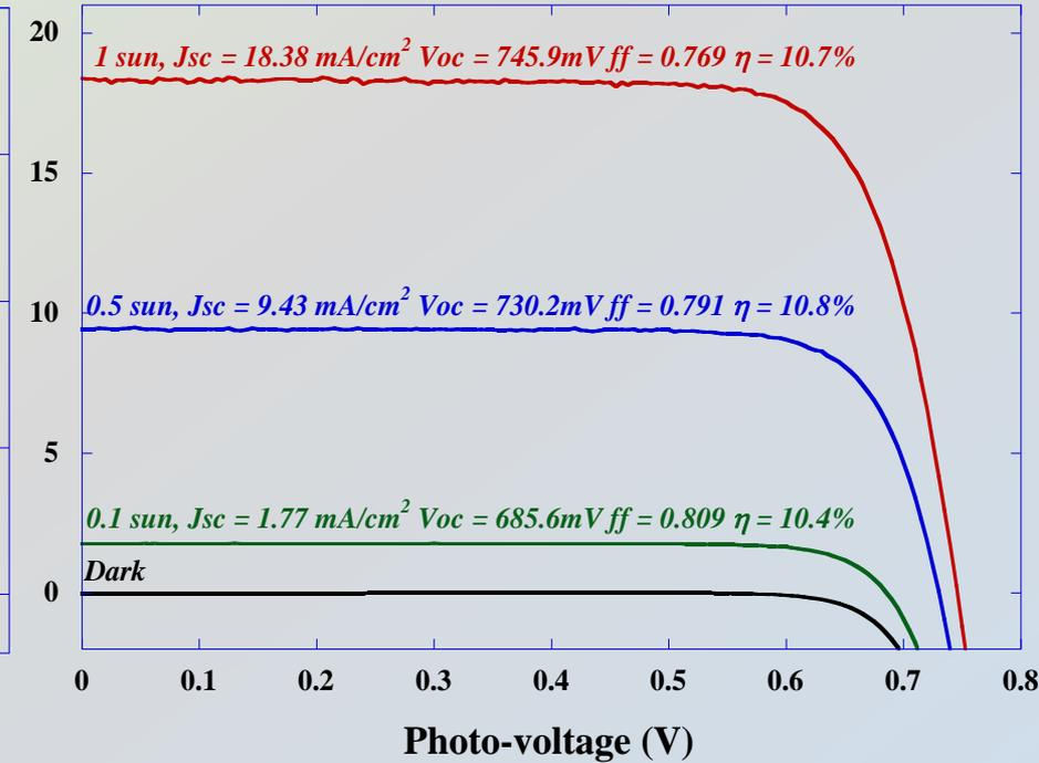
**Significant improvement of power conversion efficiency when using the beads (gain in  $J_{sc}$  and  $V_{oc}$ )**
