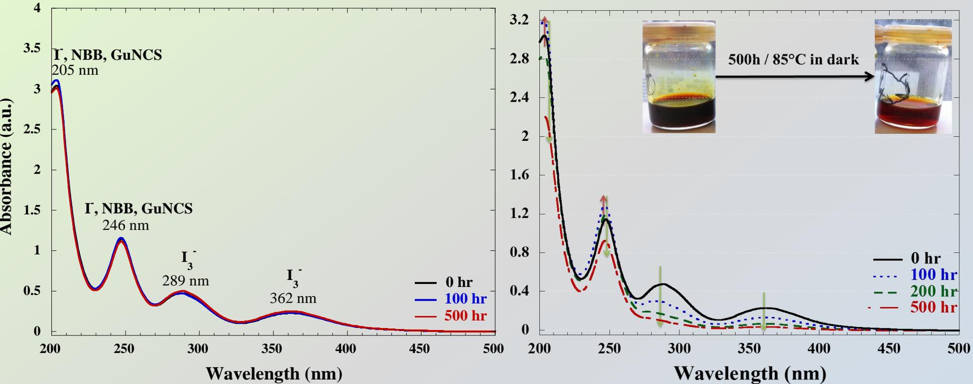
The well-known iodine depletion stems from the surface of  $TiO_2$  (activated by temperature and no light action)
