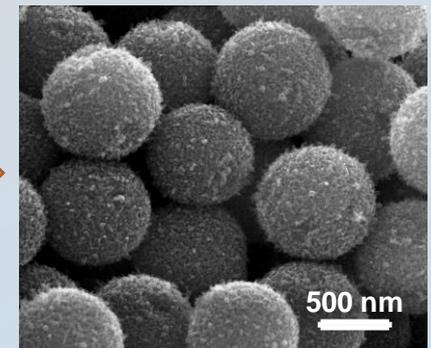
*Synthesis of bifunctional beads of  $\text{TiO}_2$*
