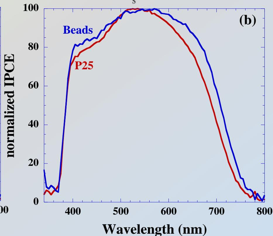
*Enhancement of light conversion in the whole absorption spectrum of the dye*
