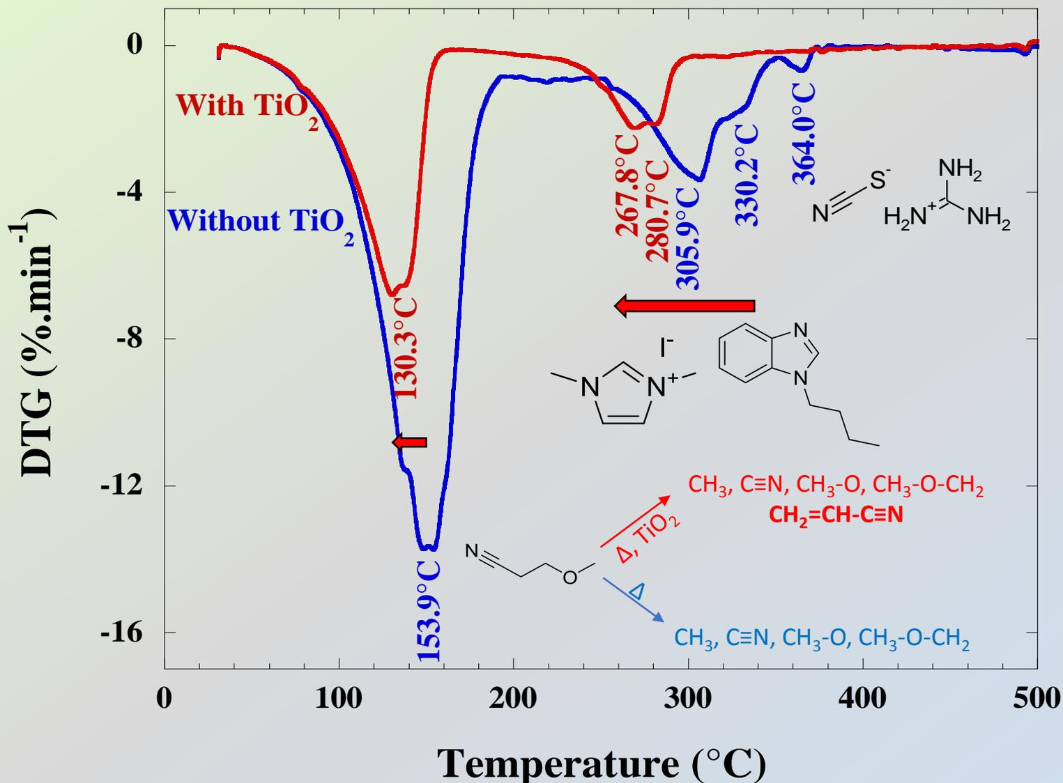
*The surface of  $TiO_2$  catalysis the thermal degradation of MPN electrolyte components and induces AN formation as an intermediate degradation product*
