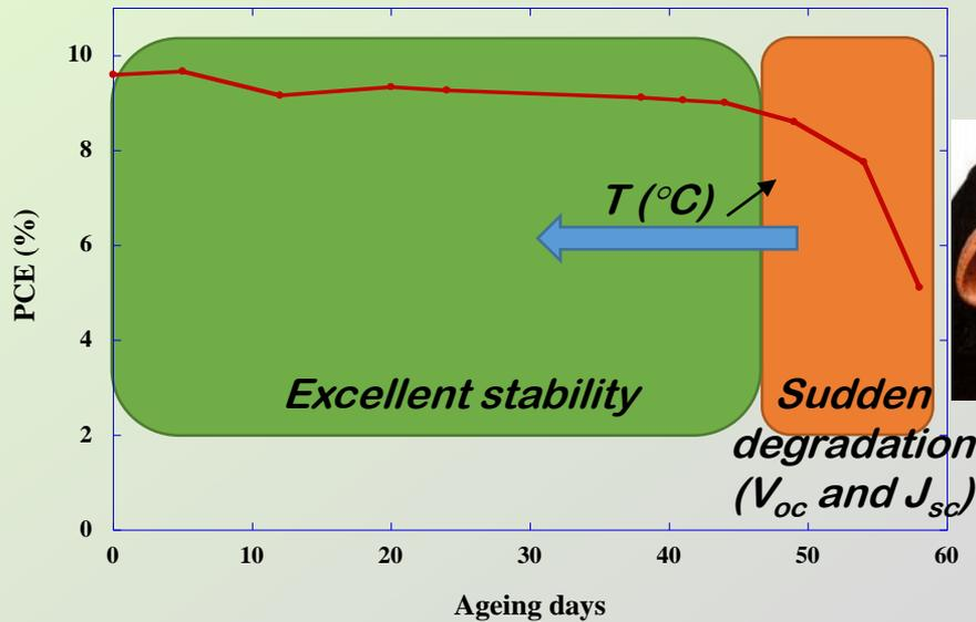
Evolution of cell ageing unusual for an electrochemical device with sudden breaking down
