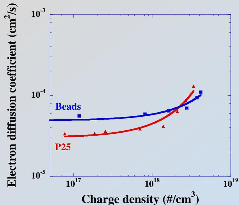
**Greater electron lifetime and enhanced charge transport in beads**
