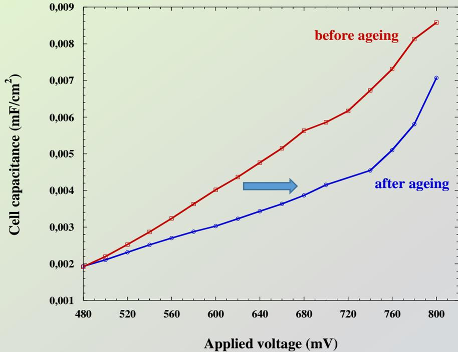
*Upshift of the surface trap states contributing to the cell capacitance*
