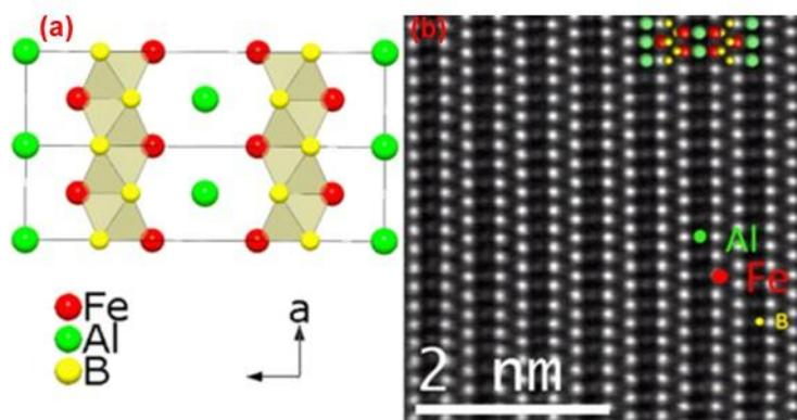
Fig.1  $\text{AlFe}_2\text{B}_2$  unit cell. (b) High-resolution HAADF STEM image of  $\text{AlFe}_2\text{B}_2$  taken along the  $[101]$  zone axis along with a projection of a unit cell represented with Fe (red), Al (green), and B (yellow) spheres [Phys. Rev. Materials 2, 084408 (2018)].
