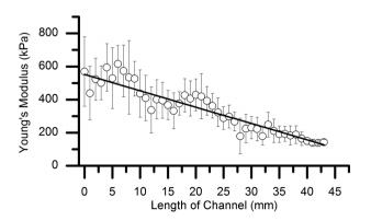
**Fig. 7** Young's modulus of PEM films with EDC gradient obtained by AFM-nano indentations. Force-indentation profiles were collected every millimeter along the length of the channels. Error bars represent the standard deviation of nine measurements performed at every point in two different channels. A slope of  $-9.90 \text{ kPa mm}^{-1}$  was obtained from a linear fit ( $R^2$  0.94).
