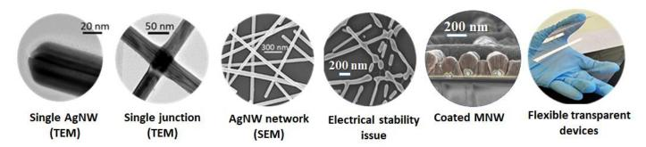
Electronic or optical pictures of AgNW, AgNW networks showing the different length scales that play a role, up to the transparent electrode devices (on the extreme right)
