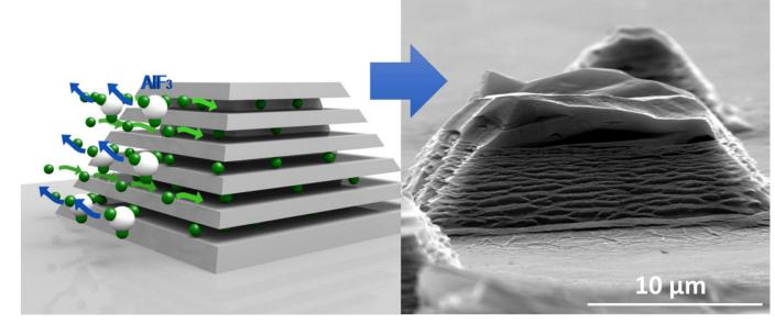
Chemical exfoliation of pillars etched from MAX phase single crystals.
