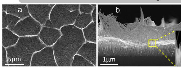
Nano-architectured long lasting superhydrophobic surface: top view (a) and cross section (b) (CEMAM Labex project)
