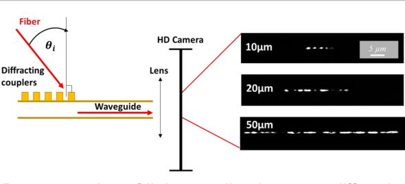
Demonstration of light coupling between diffraction gratings and channel waveguides of various width
