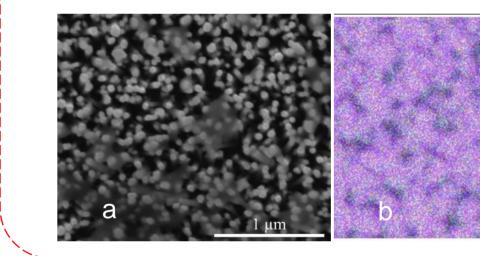
ZnO Nanowires impregnated with PDMS for water filtration applications: SEM (a) and EDX image (b). Green and violet dots represent the presence of Si and Zn, respectively (Nanoscience Foundation project)
