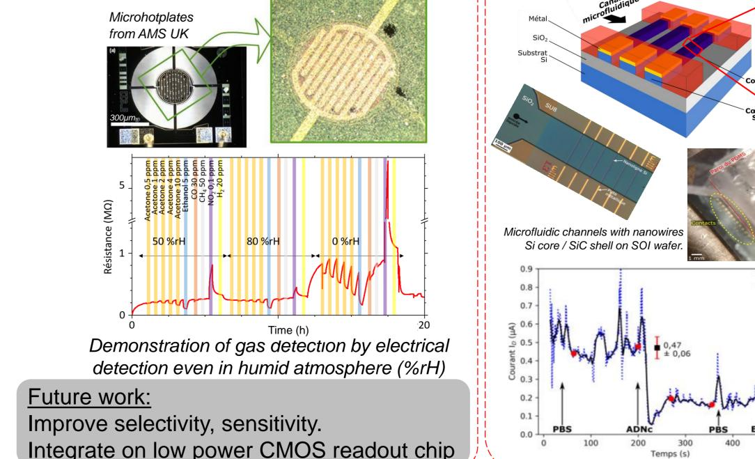
Amorphous SiC shell deposited by PECVD on Si nanowire on SOI wafer Better stability and biocompatibility of SiC towards physiological conditions than Si  $V_{D} = -4 V_{C}$  $V_{G} = -5 V_{C}$ Demonstration of electrical properties change upon DNA hybridization in liquid Future work: Improve selectivity, sensitivity and stability in vivo applications
