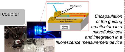
Encapsulation of the guiding architecture in a microfluidic cell and integration in a fluorescence measurement device
