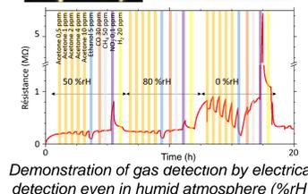
Demonstration of gas detection by electrical detection even in humid atmosphere (%RH)
