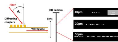
Demonstration of light coupling between diffraction gratings and channel waveguides of various width
