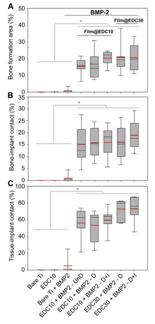
**Fig. 6.** Osteoinductive performance of the PEM-coated TA6V scaffolds. Box-and-whisker plots of (A) bone formation area given as a % of the "available area" (by subtracting the titanium scaffold surface from the whole surface), (B) bone-implant contact, given as the % of TA6V scaffold perimeter in contact to bone normalized over the Ti scaffold perimeter length and (C) tissue-implant contact in each group of TA6V scaffolds tested determined by histomorphometric analysis. \*p < 0.05.
