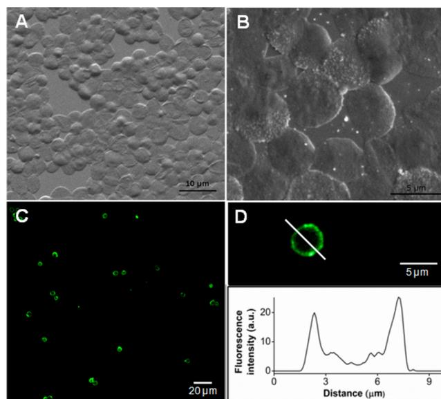
**Figure 4.** Microscopic observations of ((HA-CD-PTX)/PLL)<sub>4</sub>/HA capsules. (A, B) SEM observations of the dried hollow capsules. (C) CLSM images of capsules exhibiting a localized green fluorescence in their nanoshell resulting from the complexation of OG-PTX by CD molecules in the nanoshell. (D) Magnified image of a capsule and the corresponding fluorescence intensity profile along its diameter, confirming the selectivity of OG-PTX incorporation in the nanoshell.
