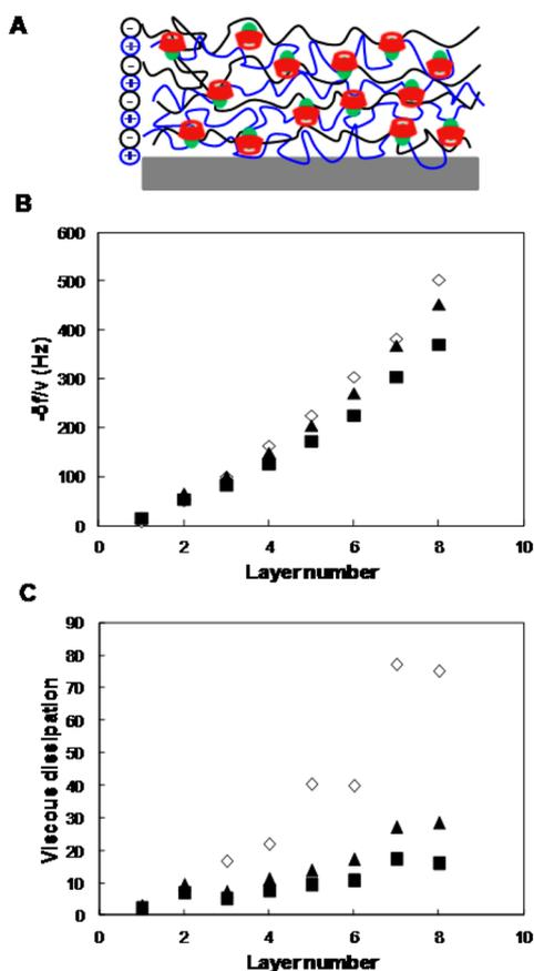
**Figure 3.** Growth of (HA-CD/PLL) films with and without PTX in 0.15 M NaCl (pH 6.5) measured by QCM-D on gold-coated crystal. (A) Schematic representation of a layer-by-layer self-assembled film of HA-CD/PLL. (B) Differences in the QCM frequency shifts measured at 15 MHz are plotted for each polyanion and PLL layer. Data are given at 15 MHz for HA-CD (■) and HA-CD-PTX (▲) as compared to unmodified HA (◇). (C) Viscous dissipations for each polyanion and PLL layer.
