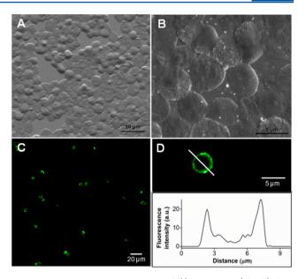
Figure 4. Microscopic observations of  $((HA-CD-PTX)/PLL)_4/HA$  capsules. (A, B) SEM observations of the dried hollow capsules. (C) CLSM images of capsules exhibiting a localized green fluorescence in their nanoshell resulting from the complexation of OG-PTX by CD molecules in the nanoshell. (D) Magnified image of a capsule and the corresponding fluorescence intensity profile along its diameter, confirming the selectivity of OG-PTX incorporation in the nanoshell.
